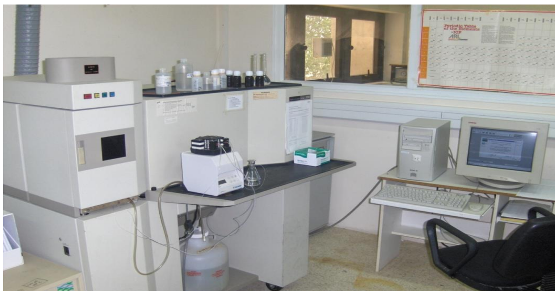
Photo 3.1: ICP-AES instrument used for heavy metals analysis
